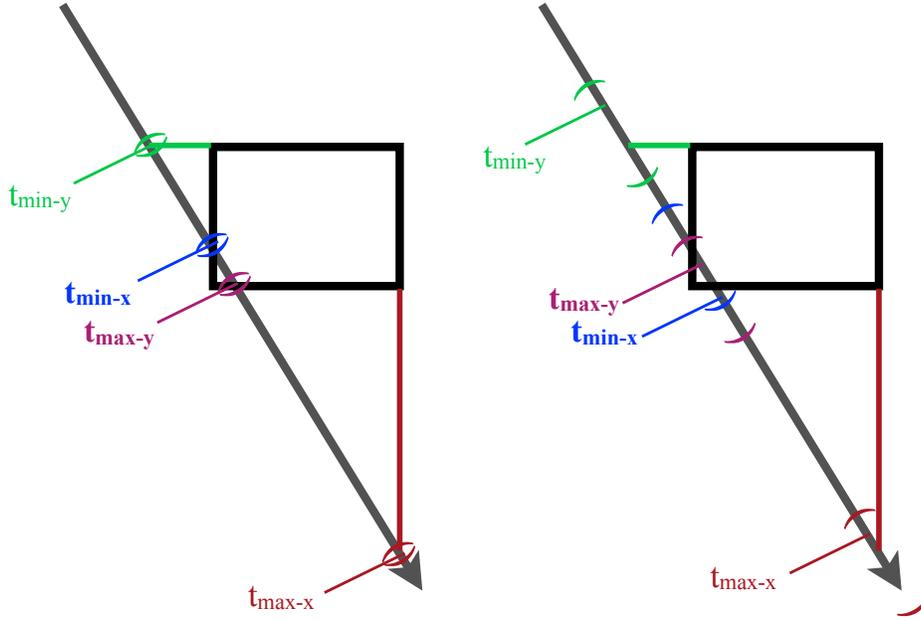
**Figure 3.** The ray is said to intersect the bounding box if the largest entry plane intersection distance,  $t_{min}$ , is smaller than or equal to the smallest exit plane distance,  $t_{max}$ . In the left example where there is no numerical error, this is the case, with  $t_{min-x} < t_{max-y}$ . However, in the right example we increase the precision error, denoted by the enlarged error bounds, and it is now possible for  $\tilde{t}_{min}$  to become larger than  $\tilde{t}_{max}$ .
