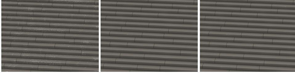
**Figure 4.** We rendered the 90.1M triangle stairs at a  $960 \times 720$  resolution with 256 samples per pixel using an ambient occlusion shader. From left to right, we used no padding of any kind, one, and then two ulps in our robust algorithm. Note that using one ulp still results in false-misses, while two ulps renders correctly without holes.
