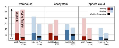
**Figure 6**. We break down the execution time of the key phases of our g-buffer control renderer, and our implementation of the visibility buffer pipeline. The scenes were rendered at 1080p resolution with eight samples per pixel. In each pair of columns, the left represents the g-buffer pipeline, the right is our pipeline. These two GPUs are comparable in their peak arithmetic throughput, making them a reasonable case study in how memory hierarchy affects rendering performance.
