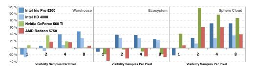
**Figure 5.** We plot the percentage speedup  $(\frac{fps_0}{fps_1} - 1.0)$  of our pipeline over the standard gbuffer pipeline as described in Section 3, for four different GPUs, three scenes, and four sampling rates at 1080p resolution. As expected, the gains are most pronounced on architectures with limited DRAM bandwidth and large cache hierarchies, and where the multisample rate is high enough that the system is bandwidth limited.
