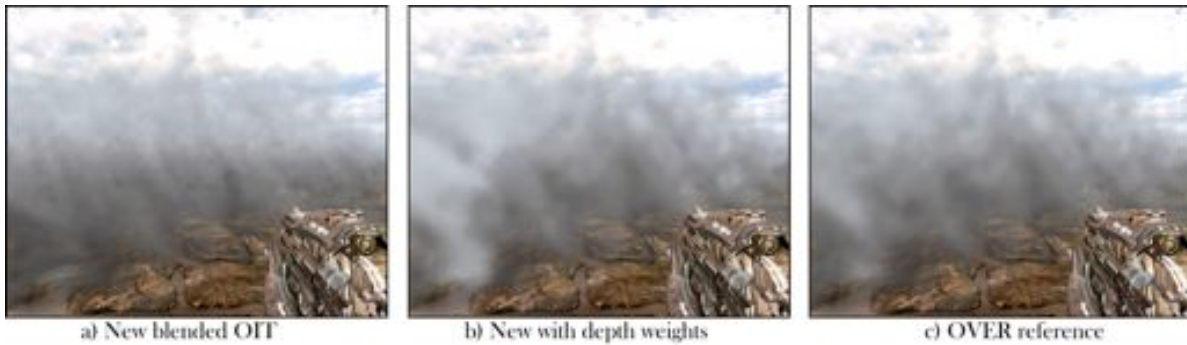
Figure 8. Smoke modeled as particles with a range of color values. Left: new blended OIT without depth weights. Right: Sorted OVER reference image.
