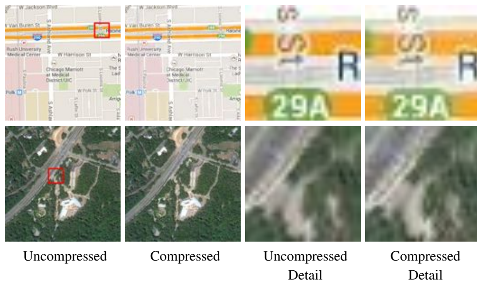
Figure 1. Texture compression using intensity dilation applied to images used in GIS applications such as Google Maps.
