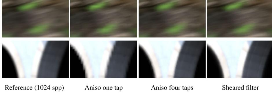
**Figure 3.** Quality of our two proposed filtering approaches. Anisotropic texture filtering works well in regions with motion (upper row), but suffers from artifacts in regions with only depth of field (lower row). We improve aniso quality by performing multiple texture lookups.
