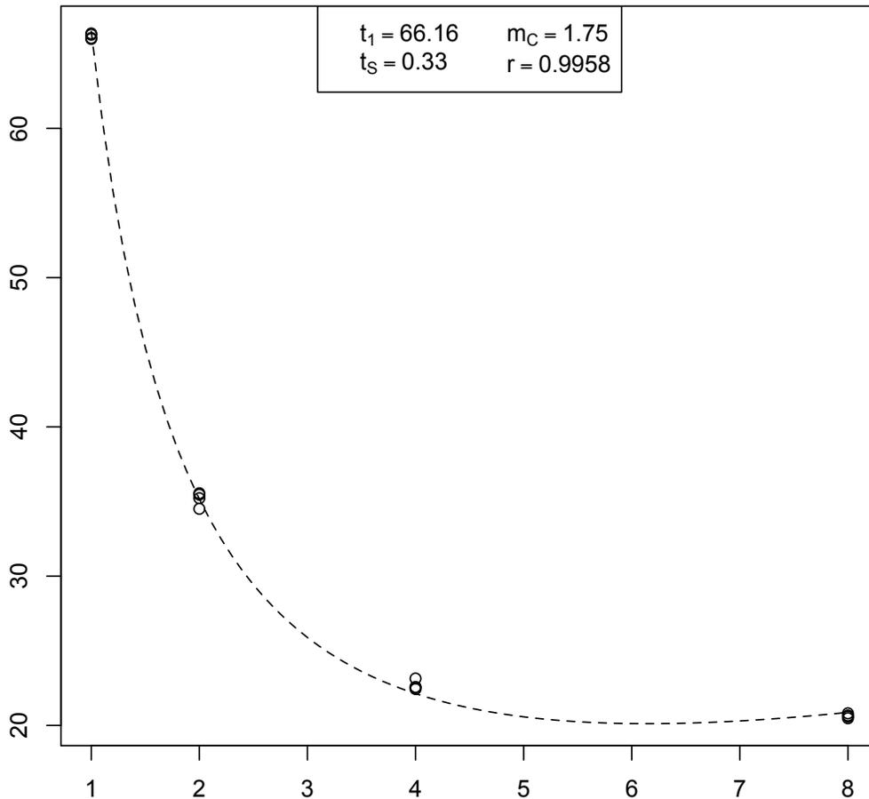
**Figure 7.** The total of merge sorting, duplicate tuple removal and  $k$ -d tree-building times (seconds) is plotted vs. the number of threads for the application of the  $O(n \log n)$   $k$ -d tree-building algorithm to  $n = 2^{24}$  randomly-generated  $(x, y, z, w)$  tuples of 32-bit integers.
