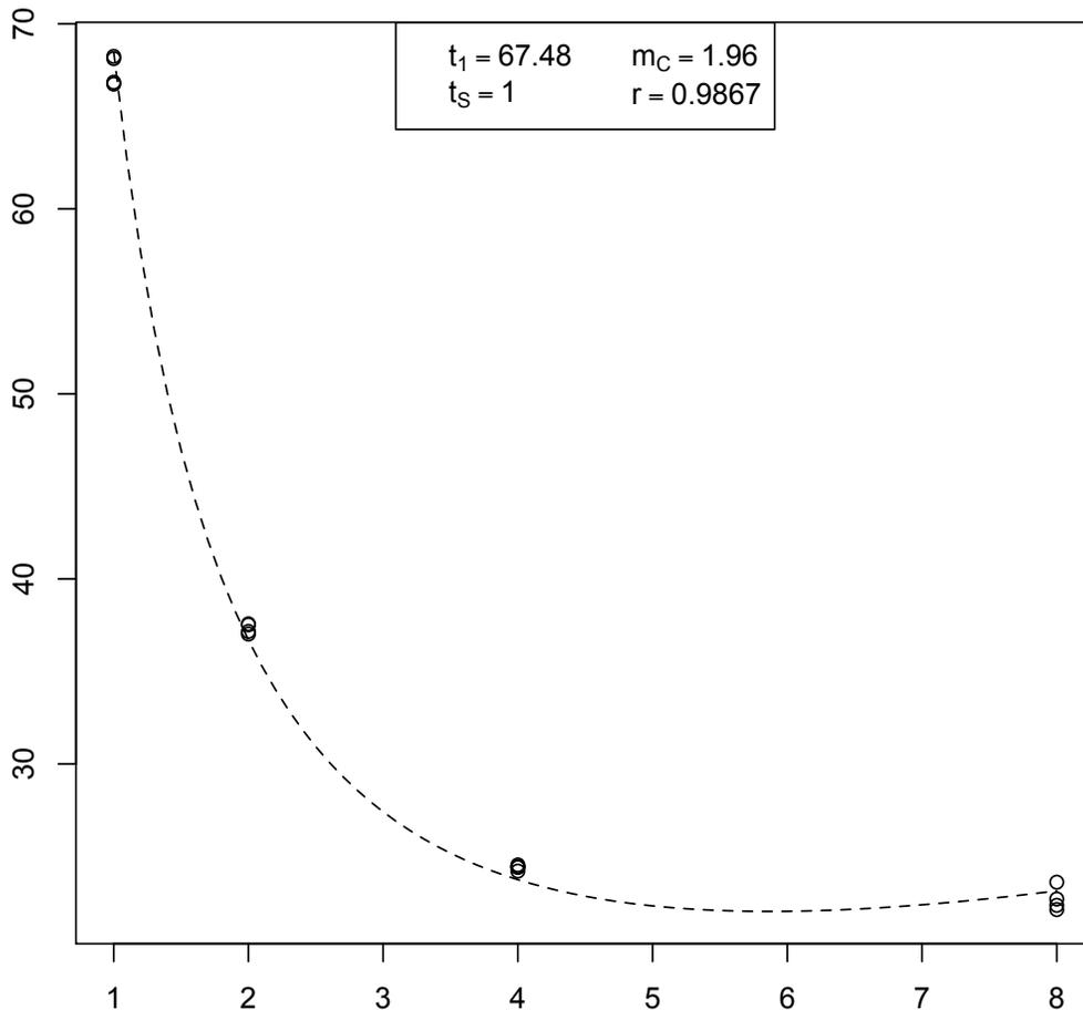
**Figure 5.** The total of merge sorting, duplicate tuple removal and  $k$ -d tree-building times (seconds) is plotted vs. the number of threads for the application of the  $O(kn \log n)$   $k$ -d tree-building algorithm to  $n = 2^{24}$   $(x, y, z, w)$  tuples of randomly-generated 32-bit integers.
