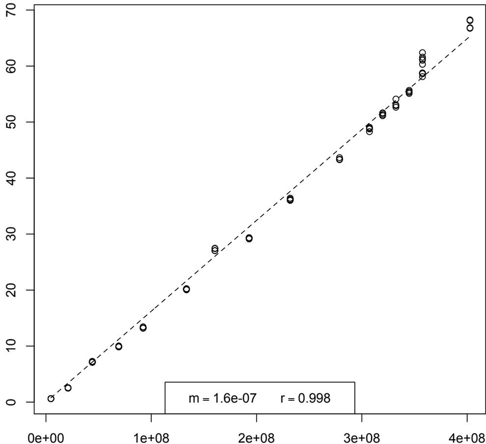
**Figure 4.** The total of merge sorting, duplicate tuple removal and  $k$ -d tree-building times (seconds) is plotted vs.  $n \log_2(n)$  for the application of the  $O(kn \log n)$   $k$ -d tree-building algorithm to  $2^{18} \leq n \leq 2^{24}$   $(x, y, z, w)$  tuples of randomly-generated 32-bit integers.
