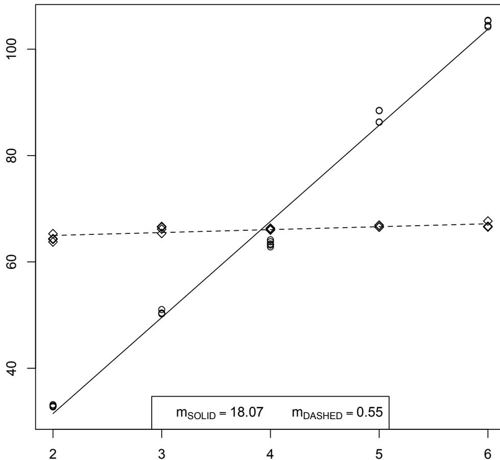
**Figure 8.** The total of merge sorting, duplicate tuple removal and  $k$ -d tree-building times (seconds) is plotted vs. the number of dimensions  $k$  for the application of the  $O(kn \log n)$  algorithm (solid line and circles) and the  $O(n \log n)$  algorithm (dashed line and diamonds) to build a  $k$ -d tree from  $n = 2^{24}$   $k$ -dimensional tuples of randomly-generated 32-bit integers.
