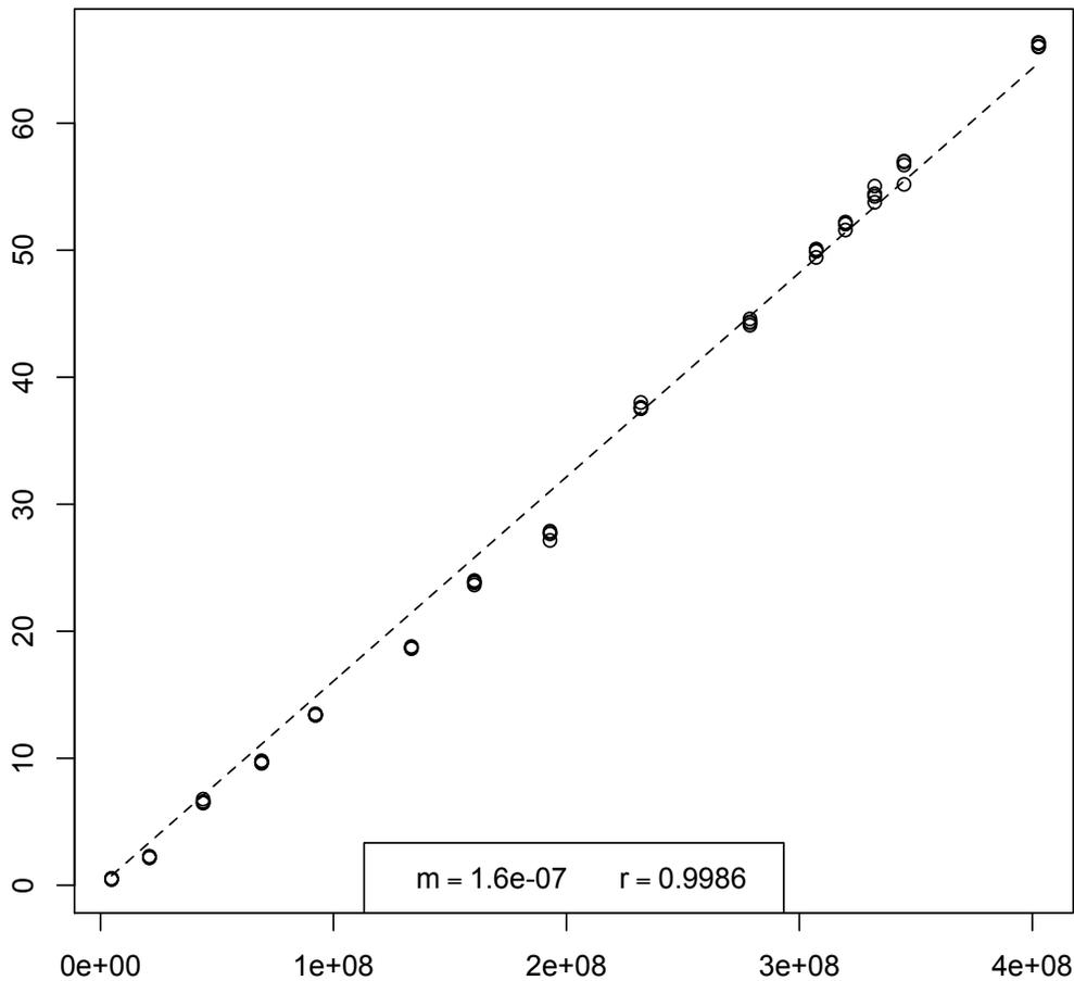
**Figure 6.** The total of merge sorting, duplicate tuple removal and  $k$ -d tree-building times (seconds) is plotted vs.  $n \log_2(n)$  for the application of the  $O(n \log n)$   $k$ -d tree-building algorithm to  $2^{18} \leq n \leq 2^{24}$   $(x, y, z, w)$  tuples of randomly-generated 32-bit integers.
