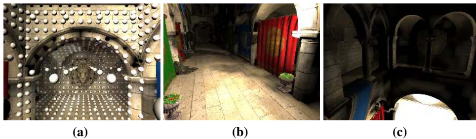
Figure 9. Possible artifacts of the algorithm. (a) Light map caches (black ones) are placed behind other geometry. This can be fixed by enabling backface culling during cache precomputation; (b) A small spotlight (top right) reveals discontinuities in linkage on the floor; (c) Single bounce light bleeding (amplified by \times 4096 ): the upper corridor should be black. The cause is that the hierarchy can merge clusters which cannot see each other.
