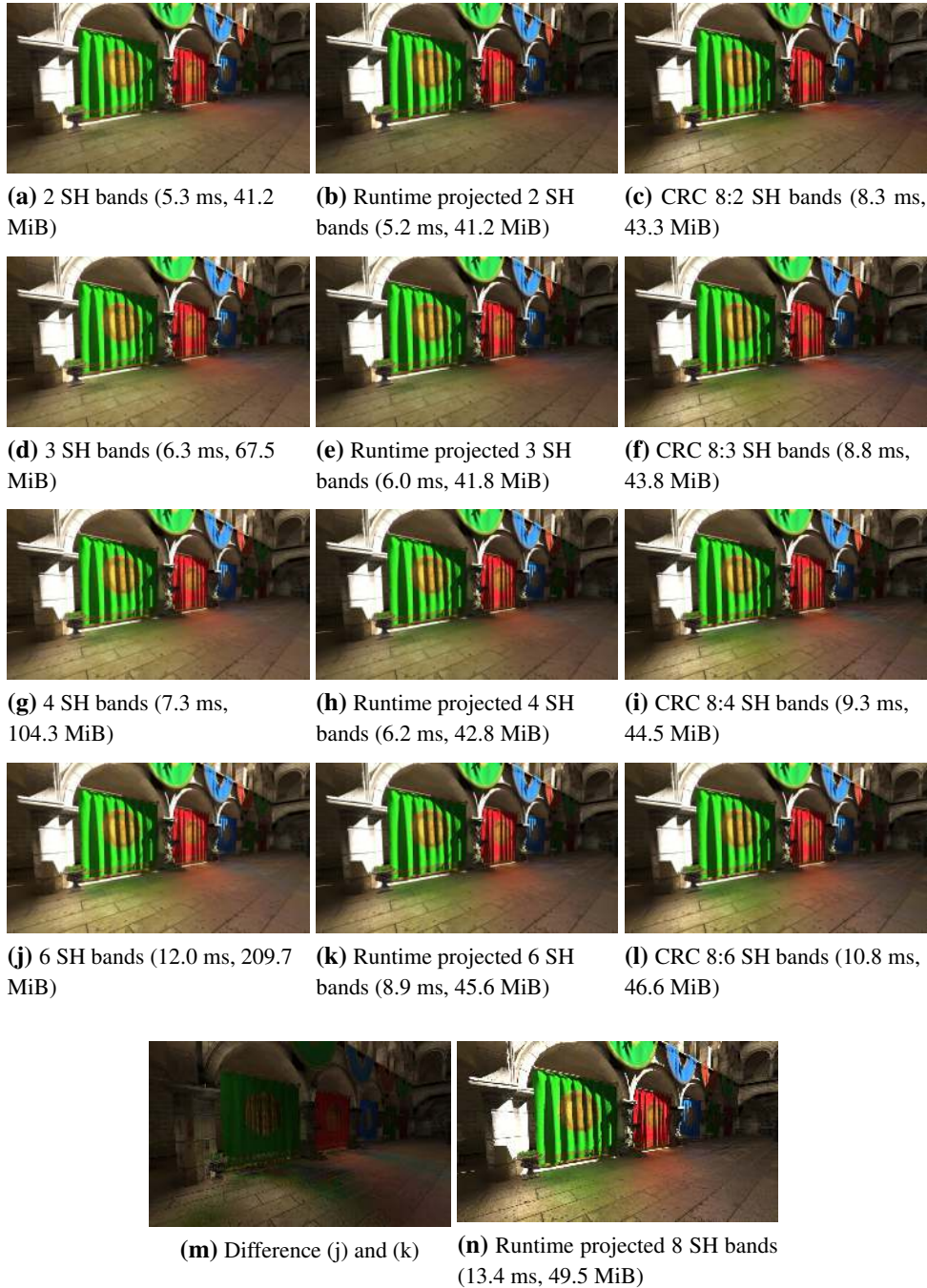
Figure 8. Glossy reflections with a Blinn-Phong-exponent of 30 at a resolution of 1920 \times 1080 with n_C = 10585 , n_L = 254 and n_S = 128k . The indirect lighting is amplified by a factor of two to emphasize the differences. The alternative implementation is similar, but not equal as the difference image (m) shows. All other difference images look very similar and are therefore not shown. Image (n) shows the results for 8 band SHs using runtime projection. Without the optimization only seven bands are possible due to the link-buffer size. The rightmost column shows the gain of chrominance compression for full eight-band runtime projection.
