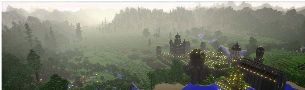
Figure 1. A massive Minecraft world rendering at 3.2 Mvoxels/ms (53 Mvoxels/frame at 60 fps) on GeForce 1080 via our fast ray-box intersection. This fully dynamic example is 7× faster than rasterization of the equivalent static mesh with precomputed visibility. The full model can be downloaded from https://www.planetminecraft.com/project/apterra---huge-custom-survival-map/ .
