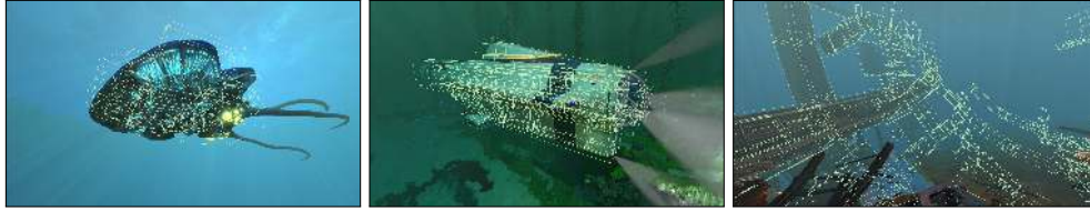
Figure 4. Oriented boxes used for collision detection against particles and projectiles in the 2018 PC video game Subnautica . A typical scene might contain millions of instanced oriented boxes for such non-rendering applications. Our ray-box algorithm is suited to this application as well as rendering. Images courtesy of and ©2018 Unknown Worlds.
