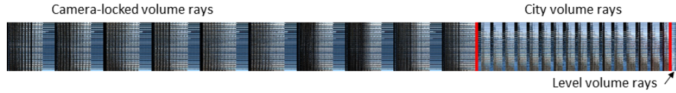
Figure 11. Shaded ray data for multiple volumes packed into a single texture. This texture is irradiance data taken from our multivolume scene in the supplemental video. The texture includes shaded update rays for the camera-locked volume, the city-scale volume, and the level-scale volume—these are labeled in the figure and delineated within the texture by the red lines (which are not part of the irradiance data).
