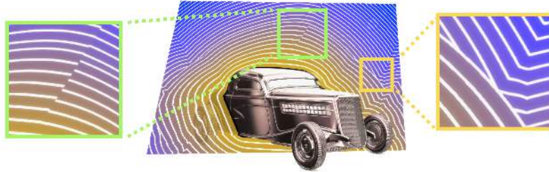
Figure 14. Detecting SDF discontinuities. Middle: A car with its SDF on a cutting plane. Left: A close-up from the center-top of the cutting plane, showing disconnected contour lines. Right: A close-up from the right side of the cutting plane, showing contours lines touching one another.
