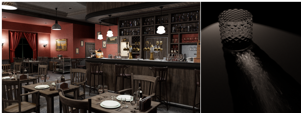
Figure 1. Two scenes rendered in less than a minute with our hardware ray traced photon mapper. Two million photons are distributed per iteration in both scenes. Left: Bistro (30 s, 2304 it, \sim 13 ms per iteration). Right: Caustic Glass (2 s, 193 it, \sim 10.4 ms per iteration). Times were captured with an NVIDIA GeForce RTX 2080 SUPER.
