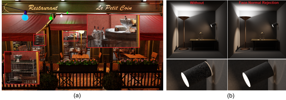
Figure 9. Both images were rendered with 2000 iterations. (a) Bistro Full scene with noticeable noise on metallic objects. (b) Veach-Bidir scene with errors introduced by the thin wall of the lamp. The bright halo on the left side is present in both collection versions. The noise on the lamp is only present for Stochastic Evaluation. Face normal rejection fixes both the halo and the noise.
